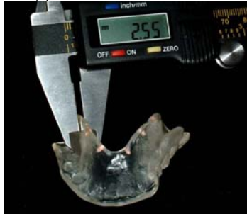
Proper thickness of guide
